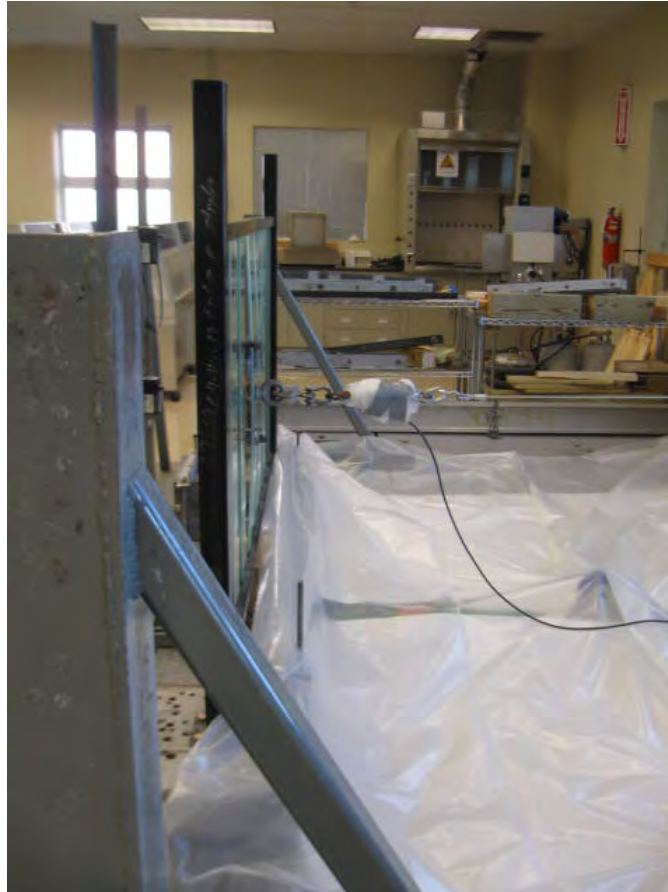
Photo No. 3 In-Fill Load Test at Center of Two Glass Balustrades
