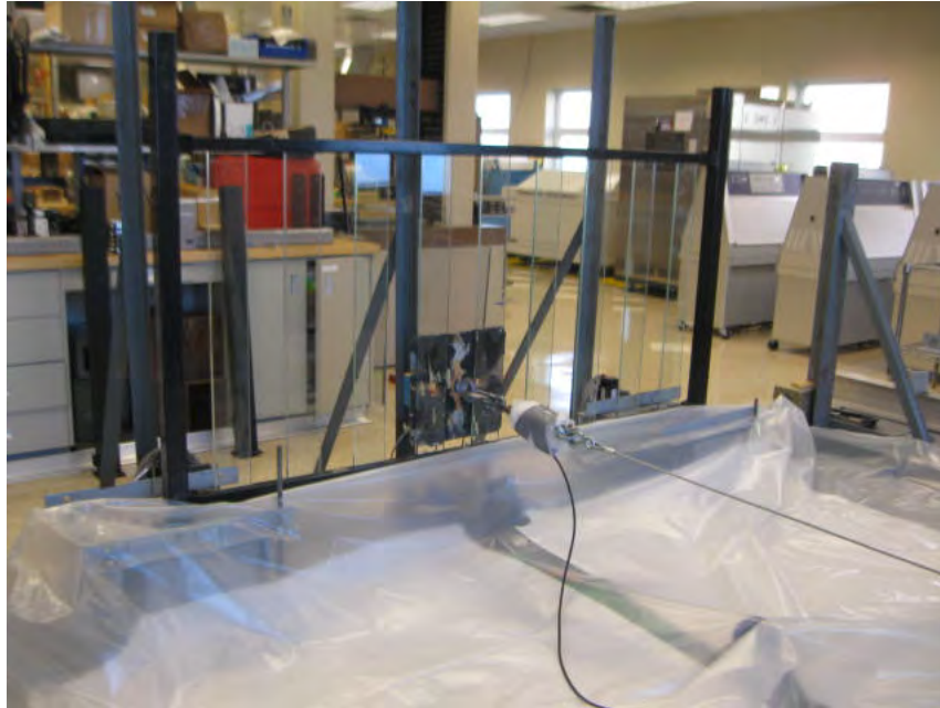
Photo No. 4 In-Fill Load Test at Bottom of Two Balustrades
