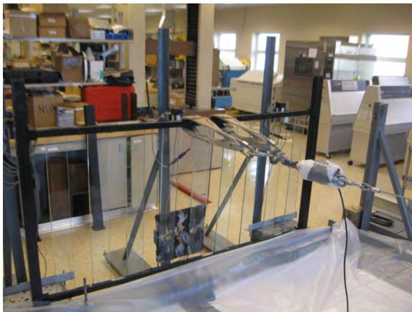
Photo No. 5 Concentrated Horizontal Load Test at Midspan of Top Rail
