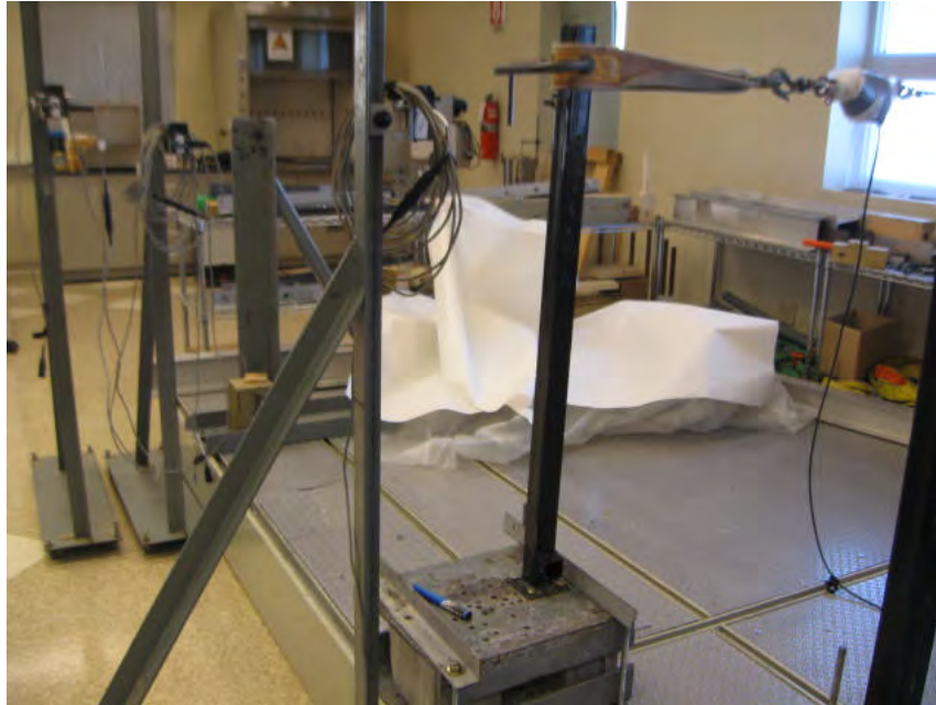
Photo No. 8 Stand-Alone Post Test with Load Applied at 42 in High
