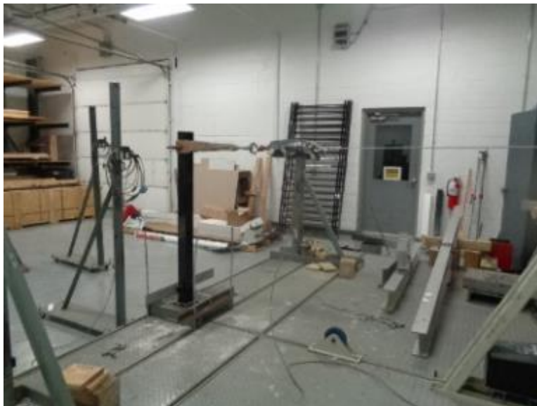
Photo No. 8 Concentrated Load at Top of Stand-Alone Post Mount
