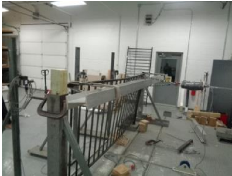
Photo No. 7 Concentrated Load Test at Ends of Top Rail (Brackets)
