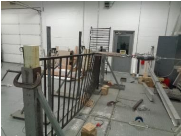
Photo No. 6 Concentrated Load Test at Mid-Span of Top Rail
