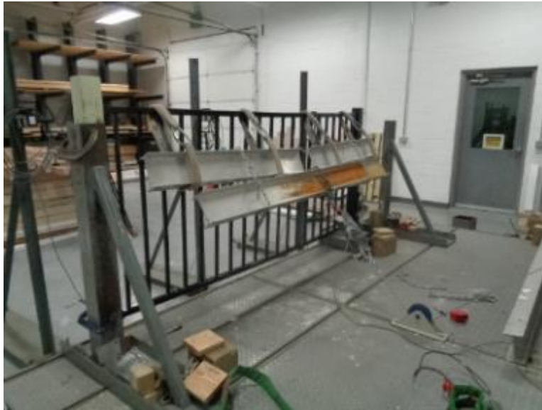
Photo No. 5 Uniform Load Applied at a 45 degree angle
