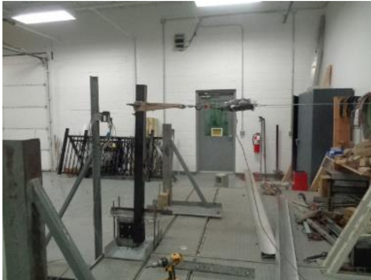
Photo No. 2 Concentrated Load Test at Top of Post Mount at 42 in
