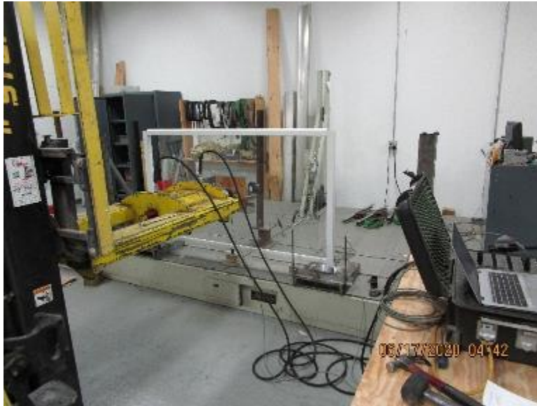
Photo No. 3 In-Fill Load Test at Center of Glass Panel
