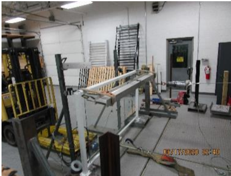
Photo No. 9 Concentrated Load Test at Ends of Top Rail (Brackets)
