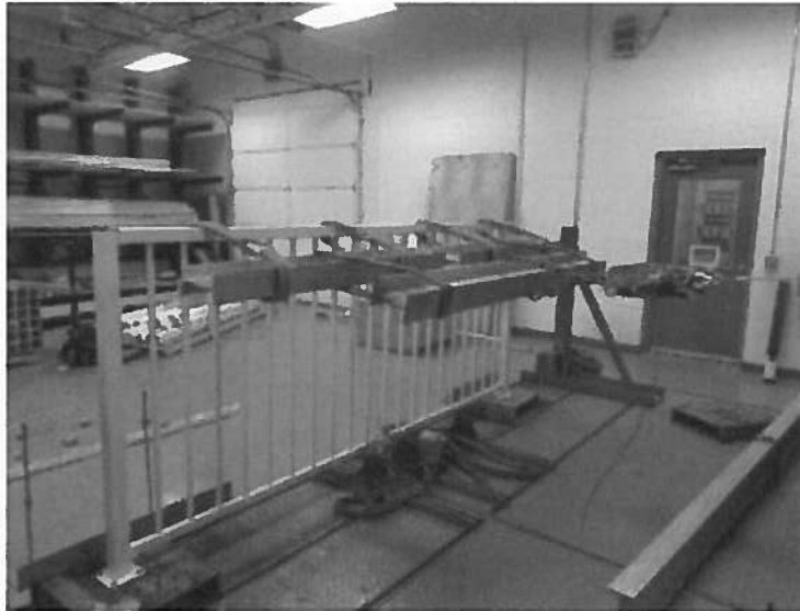
Photo No. 7 Horizontal Uniform Load on Top Rail
