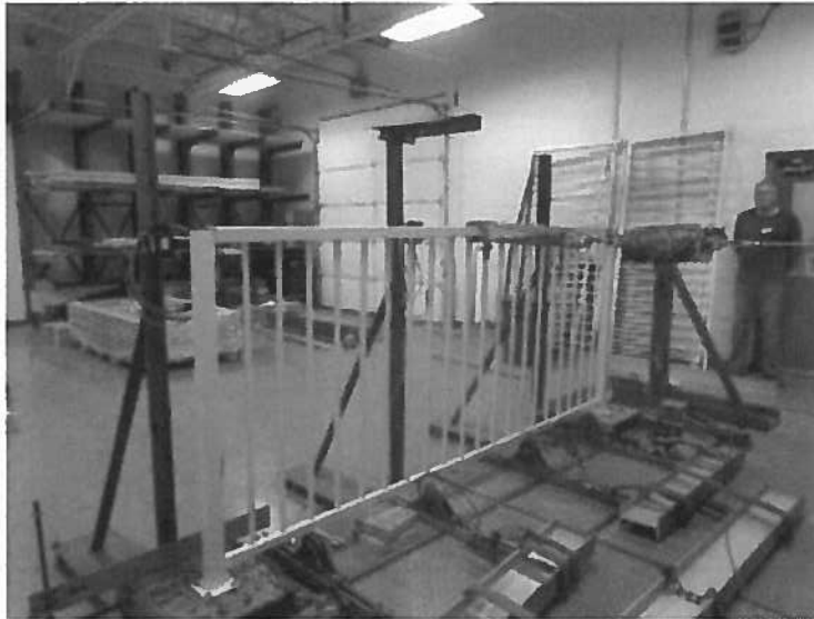
Photo No. 3 Concentrated Load Test at Midspan of Top Rail
