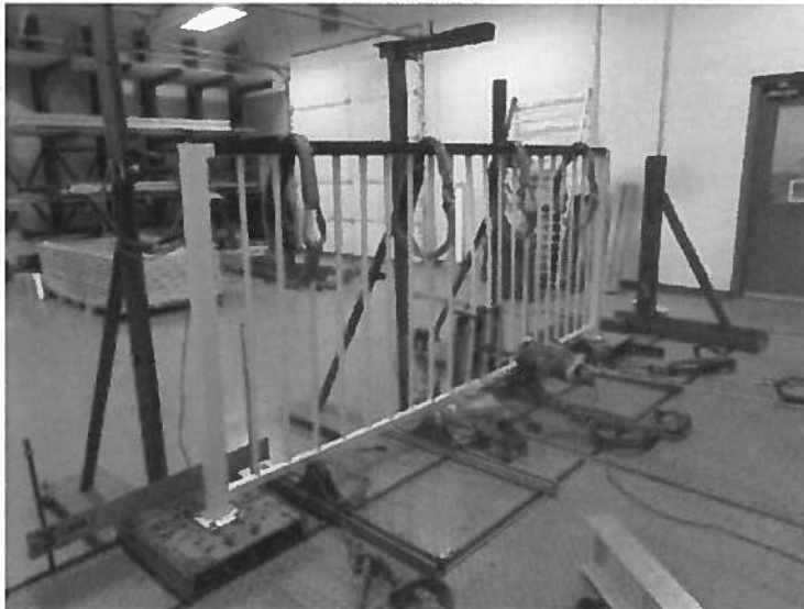
Photo No. 2 In-Fill Load Test at Bottom of Three Pickets
